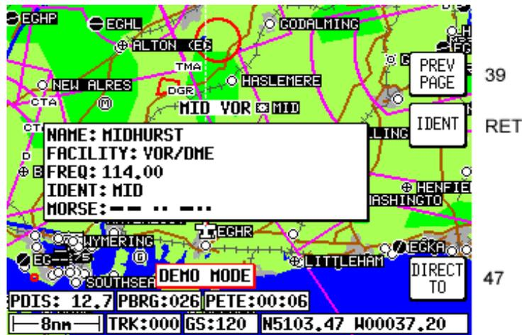
This screen times-out back to the previous screen if joystick not moved or key is not hit for 30 seconds
