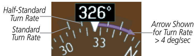
Figure 2-19 Turn Rate Indicator and Trend Vector
