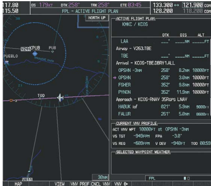
Figure 5-131 Approaching Top of Descent (TOD)
